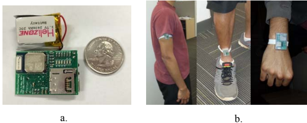
Fig. 4. Left: IMU Sensor Used, Right: Body sensor placements
