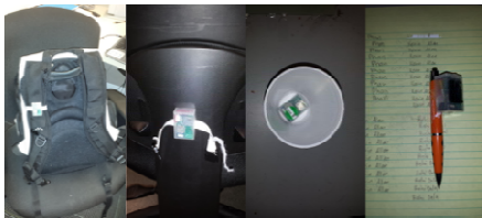
Fig. 5. Object sensor placements from left to right: sensor on backpack, sensor on chair, sensor in cup, sensor attached to pen
