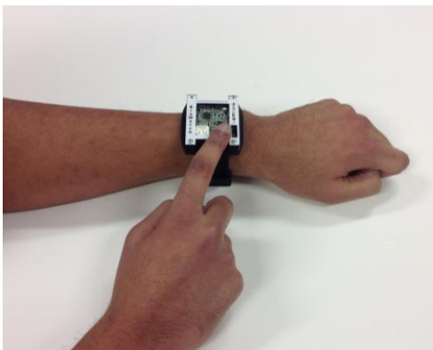
Fig. 1: BioWatch with two electrodes underneath the watch making contact with the left arm and the top electrode making contact with the right arm via a finger touch.
