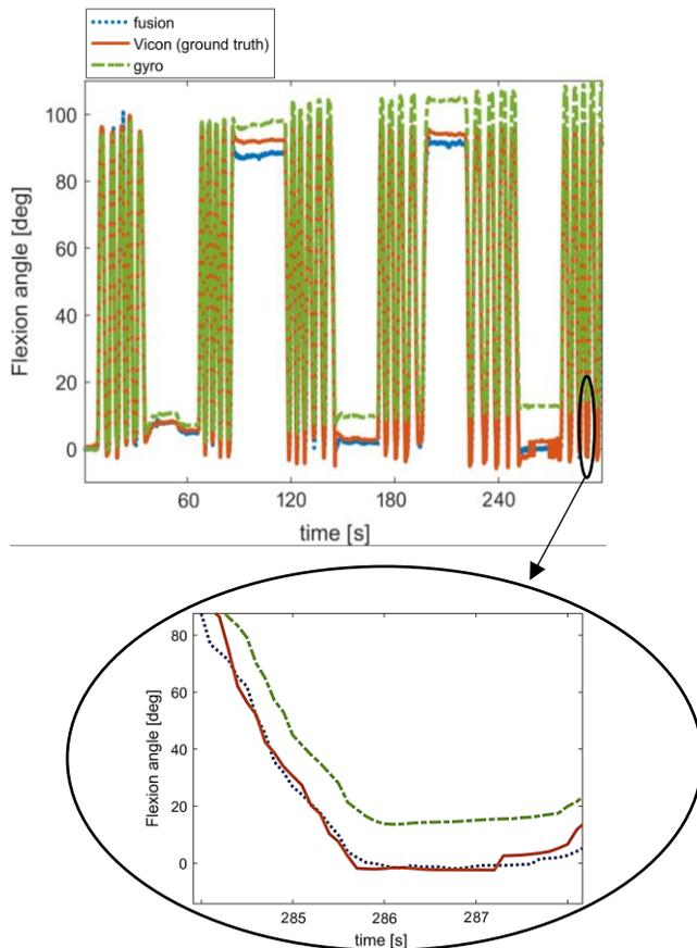
Figure 3 –long-term arm flexion and drift effect on gyroscope
