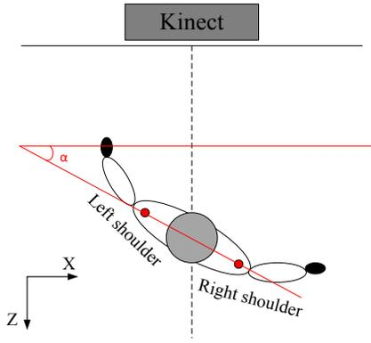
Figure 2 – The angle between the two shoulders when occlusion occurs
