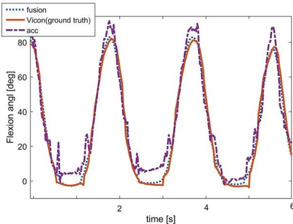
Figure 4 - Thigh high acceleration flexion and its effect on accelerometer. Accelerometer angle has big error in the beginning and end of movement (peaks and valleys)
