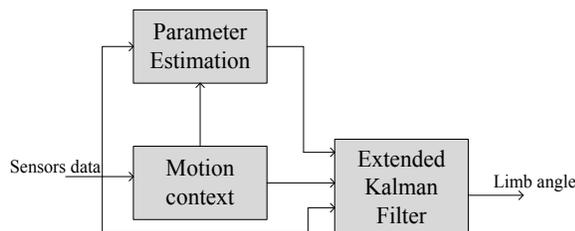
Figure 1 – Block diagram of the proposed system
