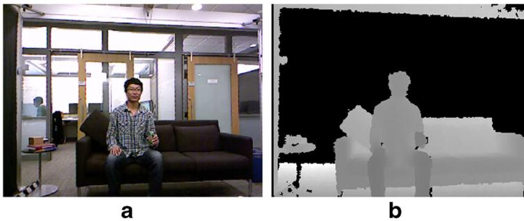
**Fig. 2** **a** An example color image ( $640 \times 480$ ) from the MSR Daily Activity 3D dataset [65], **b** corresponding depth image ( $320 \times 240$ )
