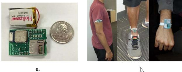
Fig. 4. Left: IMU Sensor Used, Right: Body sensor placements
