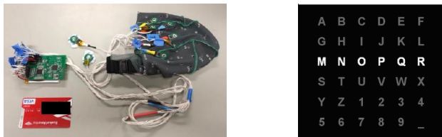
Fig. 1A (left) EEG data acquisition system B (right) P300 speller matrix with one row intensified
