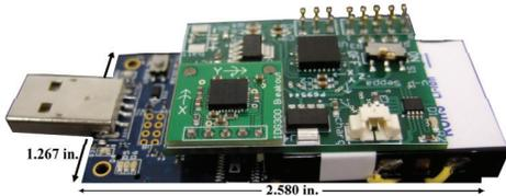
Figure 1: Mote with inertial sensors
