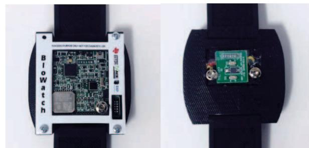
Fig. 2: BioWatch (front and back) designed in our lab
