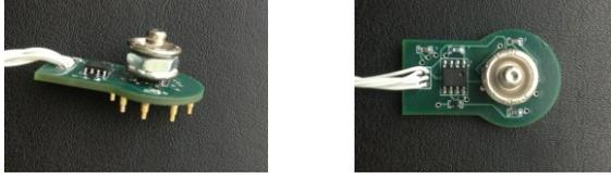
Figure 2 – MUX Electrode front and back
