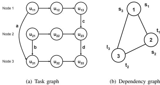
Fig. 4. A task graph and corresponding dependency graph for a network of three nodes. Dependencies shown by inter-node edges  $a$ ,  $b$ ,  $c$ , and  $d$  in the task graph are translated into the set of node pairs  $(s_k, t_k) = (1, 2), (2, 3), (1, 3)$ .
