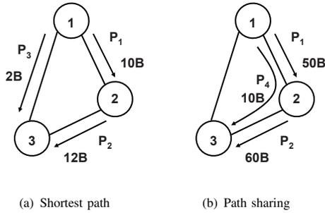
Fig. 2. Transmission using shortest path, and path sharing.
