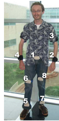
Fig. 2. Experimental subject wearing eight sensor nodes.
