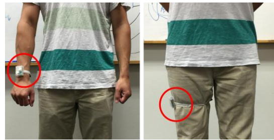
Fig. 5. Inertial sensor placements: right wrist or right thigh.
