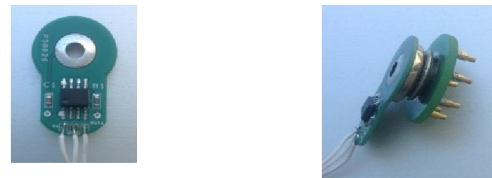
Figure 3 – (left) Electrode snap with buffer circuit (right) attached to finger based dry electrode
